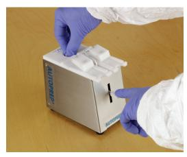
Once the smear control knob is adjusted to produce the desired thickness of smear, it is generally not necessary to make further adjustments except for specimens having extremely high or low hematocrits. However, each user should independently assess their own needs for quality smear preparation and adjust accordingly.
