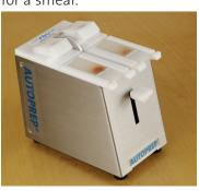
**STEP 4**- After the timed pause (approximately 2-3 seconds) to let the blood spread laterally and "wet" the glass blades side to side, the spreaders then pull the blood gently along the slide. Remove slides, prepare for staining and review.
